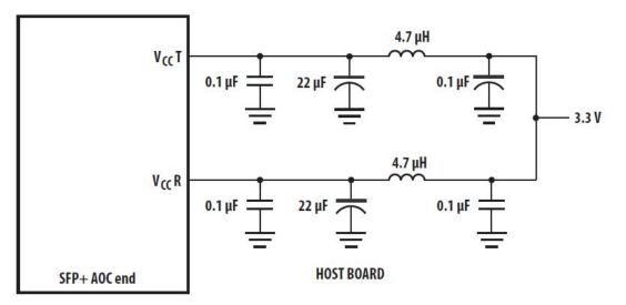
NOTE: INDUCTORS MUST HAVE LESS THAN 1 $\Omega$  series resistance to limit voltage drop to the SFP module.
